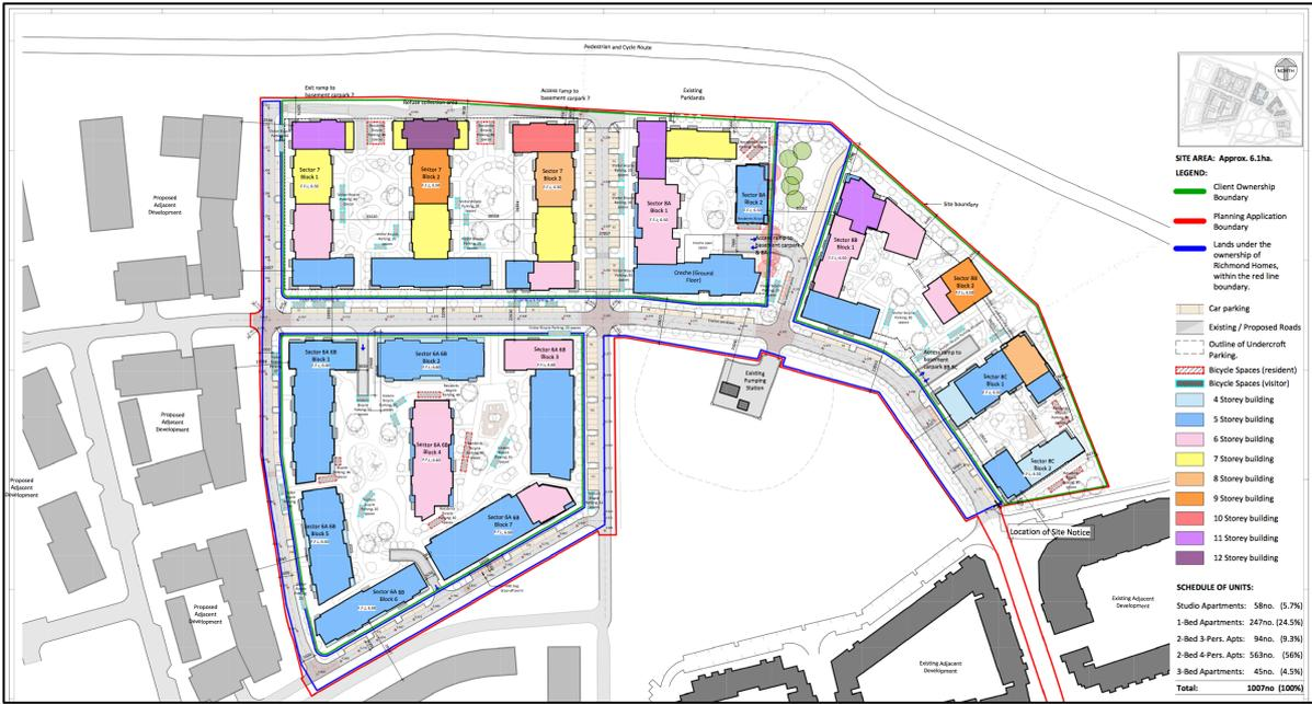
Figure 2: Extract from Drawing BALN5 -CCH -00 -ZZ -DR -A -015, indicating the location of the proposed buildings which may contain PV panels
