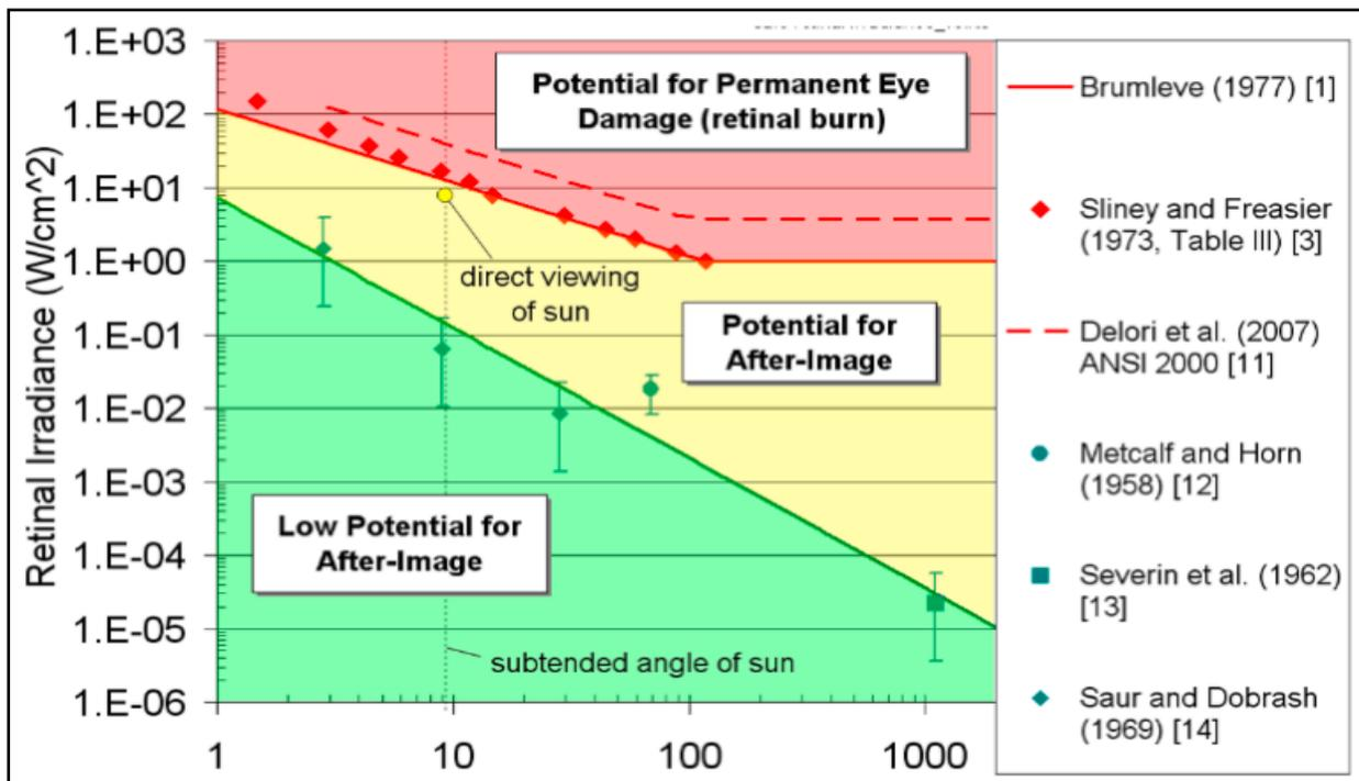
Solar Glare Ocular Hazard Plot: The potential ocular hazard from solar glare is a function of retinal irradiance and the subtended angle (size/distance) of the glare source. It should be noted that the ratio of spectrally weighted solar illuminance to solar irradiance at the earth’s surface yields a conversion factor of ~100 lumens/W. Plot adapted from Ho et al., 2011.
